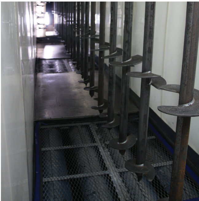
FIGURE 6-6 : Helical Lead Sections Hung From Conveyor System
