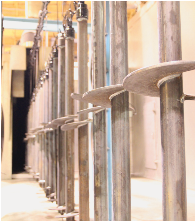
FIGURE 6-7 : Helical Lead Sections Leaving Shot Blast Cabinet
