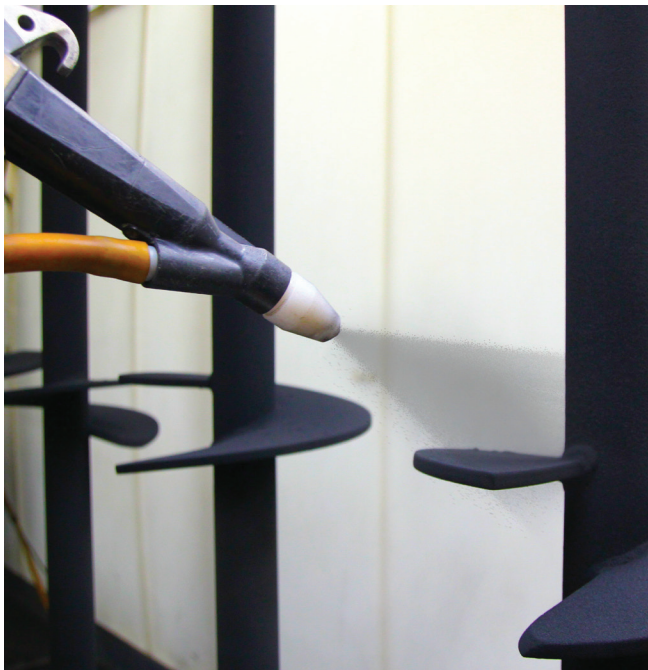
FIGURE 6-8 : Application of Powder Coating
