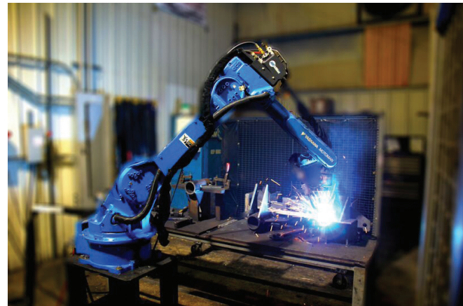
FIGURE 1-4 : Ram Jack Robotic Welder
